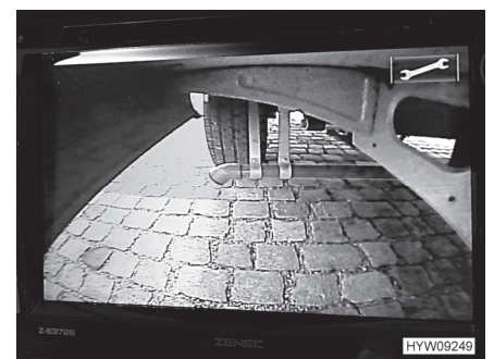
Fig. 35 Display of the waste water tank camera (example)
