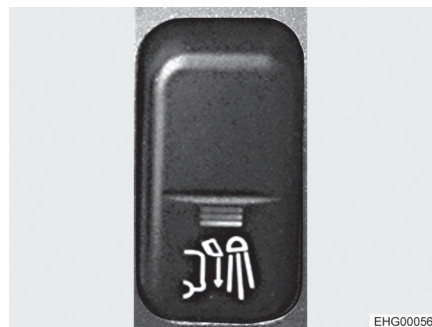
Fig. 43 Rocker switch (rear area lighting)
