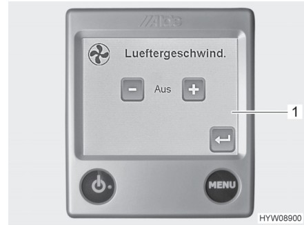
Fig. 167 Control (auxiliary fan)
