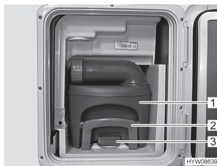
Fig. 203 Sewage tank (in the vehicle)
