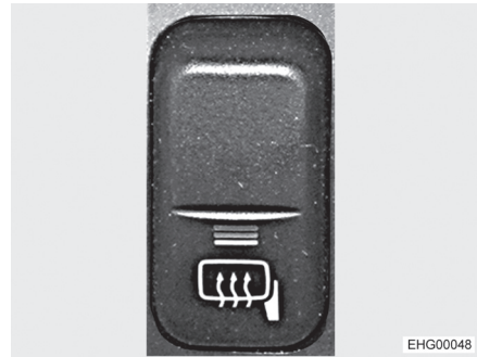
Fig. 32 Switch (mirror heater)
